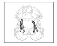
• Check the condition of the elastic and/or plastic keepers (e.g. cuts, wear, tears).
