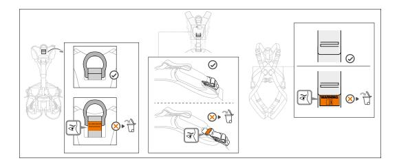
• On the European version of the VOLT harnesses: check the stitching on the LADDER CLIMB attachment-point strap.
