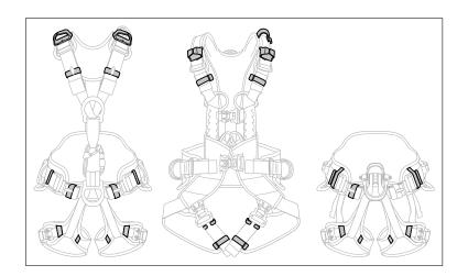
• Check the condition of the equipment loops (e.g. cuts, wear, tears).
