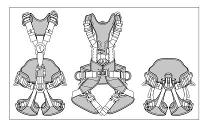
• Check the condition of the leg loop elastic bands (e.g. cuts, wear, tears).
