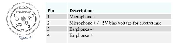
The headset connector is a 4-pole male XLR connector and supports mono headsets with electret or dynamic microphones, depending on menu settings.
