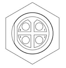
Pin 1: Power (+) Pin 2: Data Pin 3: CLK (clock pin) Pin 4: Power (-)
