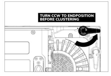
3. Make sure that the C-Lok hooks are turned counterclockwise (CCW) to the end-position first before you finally lock the C-Loks.
