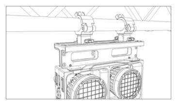
Max. Tension Load: 72kg Max. Torsion Load: 6.326 Nmm
