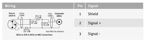
This method brings impedance matching and level matching, but no source-receiver isolation. Use a resistor network to passively attenuate the XLR signal from 3.1 V down to 0.42 V and change the impedance from 110  $\Omega$  to 75  $\Omega$ .
