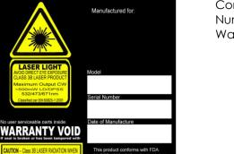
Combo label with the Product Model Number, Serial Number, Date of Manufacturing, Laser Light Warning Label, Warranty Void Label and Interlocked Housing Label
