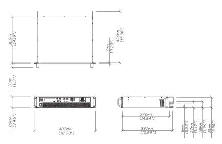
The iK42/iK81 Series Amplifier system is designed to be mounted in a standard 19" rack enclosure.
