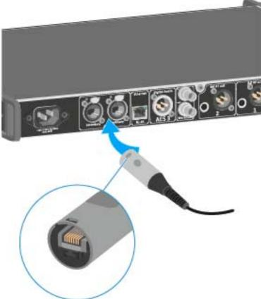
We recommend using an Ethernet connector as shown in the figure.
