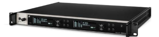
The digital 2-channel receiver works via a switching bandwidth of 244 MHz (470 to 714 MHz) that is covered by three transmitter versions (470 to 558 MHz, 550 to 638 MHz and 630 to 718 MHz). For larger 4-channel systems, you can cascade up to EM 6000s without using additional antenna splitters and you then require only one pair of antennas.
