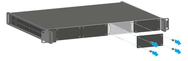
▶ Fully slide the charging module into the open charging slot as shown in the figure.
