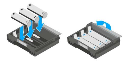
To insert the B 61 battery compartment into the SK 6000 bodypack transmitter:
