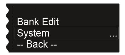
• On the display for the channel **CH 1**, the **system settings** for the whole device are also displayed in the operating menu. See "System menu item".
