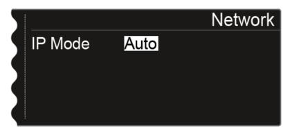
• **IP Mode mDNS**: If you use mDNS for device identification on the network, you can manually set the IP address, netmask, and gateway.
