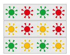
Flashing green/red >> rechargeable battery not inserted.
