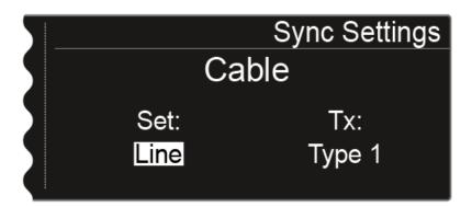
The **Cable** function is a cable emulator that you can in 3 stages (**Type 1**, **Type 2**, and **Type 3**). Cable emulation is switched off with the **Line** option.
