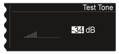
While the test tone is played back, the transmitter audio signal is muted.
