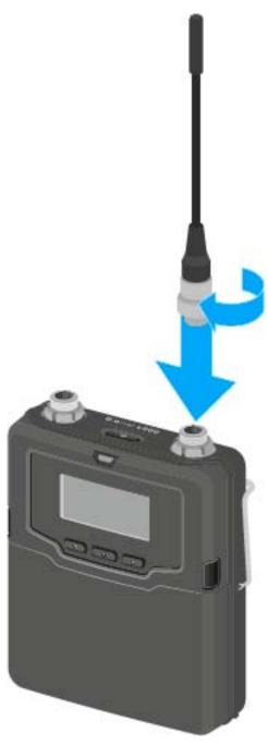
The antenna can be connected to the antenna socket very gently in only one direction. Do not use force to connect the antenna to the bodypack transmitter antenna socket.
