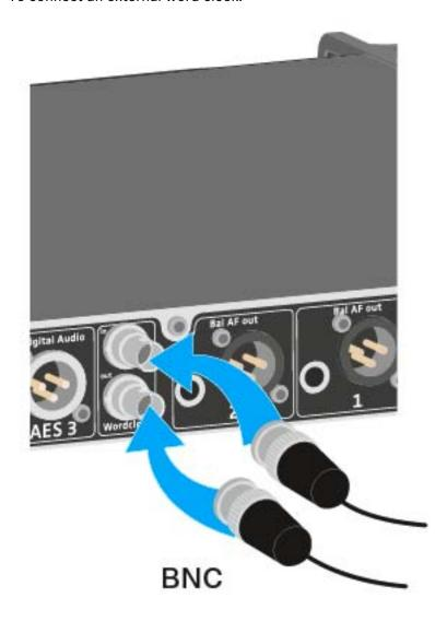
$\, \triangleright \,$  Use a coaxial BNC cable (75  $\, \Omega )$  to connect the external word clock to the Wordclock In input.
