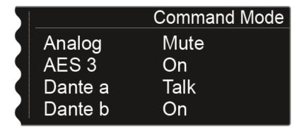
The **Analog** output signal is transmitted through the PA system for the audience. If the Command button on the transmitter is pressed, the signal on the PA system is muted. The signal is then activated on the **Dante a** channel on the Dante $^{\text{TM}}$  network. The sound technician can then hear the signal for directional instruction.
