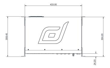
CDM32 - without box Width - 481.6mm/19" Depth - 309mm/12.2" Height - 221mm/8.7"/5U Weight - 10kg/22lbs
