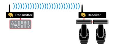
Point to multipoint operation: In this mode, one W-DMX transmitter (W-DMX TX) is communicating with up to 48 W-DMX receivers (W-DMX RX).
