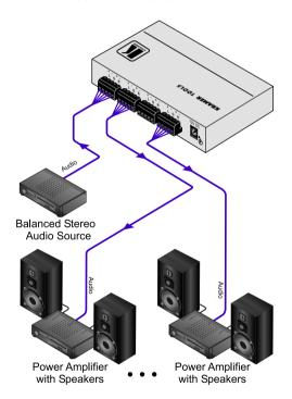
Figure 4: Connecting the VM-3AN Audio Distributor
