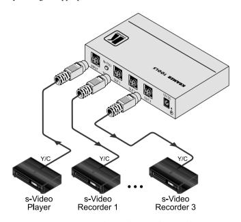
Figure 5: Connecting the VM-3SN s-Video Distributor
