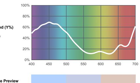
Light transmitted (Y%) for each colour wavelength (nm)
