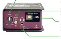
LEVEL: Used to adjust both the main stereo and headphone output signal levels.
