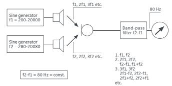
Difference frequency test set-up
