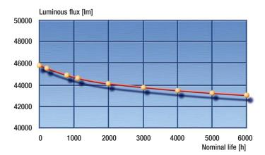
Uniform luminous efficiency throughout the life of the lamp (< 10% decline in luminous flux over its service life): 4ArXS HSD<sup>®</sup> 575W/UL/75
