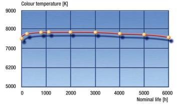
Stable colour temperature throughout the life of the lamp 4ArXS HSD® 575W/UL/75 Typical curve of colour temperature over the average life
