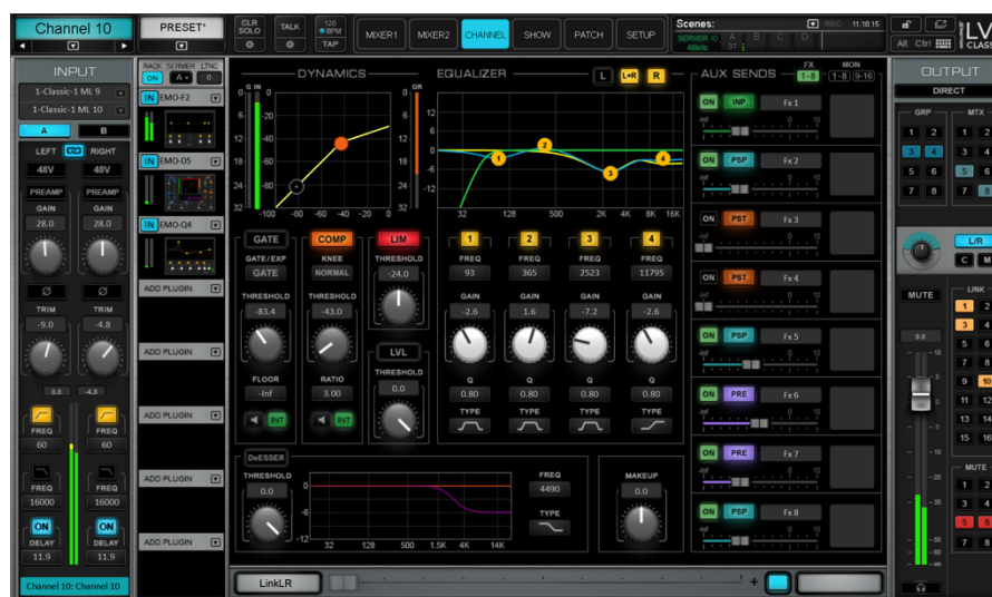
Channel window Main Control section
