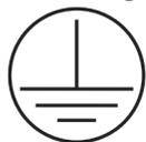
**CLASSE DE PROTECTION 1 - L'APPAREIL DOIT ÊTRE CORRECTEMENT MIS À LA TERRE**
