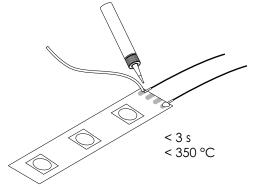
Do not solder for a period longer than 3 seconds. Make sure that the soldering temperature is lower than 350  $^{\circ}$ C.
