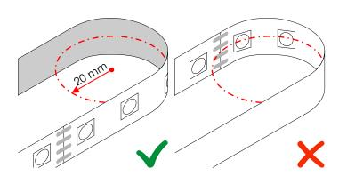
You can bend the LED strip only along the vertical axis. The minimum bending radius is 20 mm
