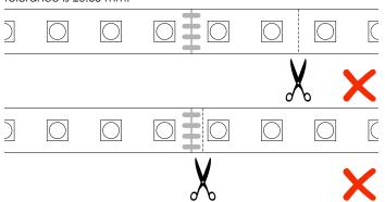
Do not cut the LED strip at any other place. This will damage the internal circuit and the LEDs will not work.
