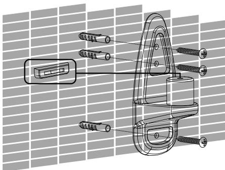
Use a pencil to mark the place for mounting. Make sure the wall structure can support the weight of monitor along with the mount. Avoid electricity for mounting holes.
