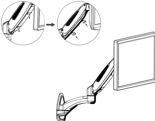
Insert cables into cable covers. Leave enough slack of cables at arm joints for full adjustment.
