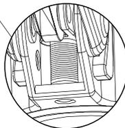
Check the screw thread. Adjust the screw clockwise, the thread becomes longer, and the load is lighter. Adjust the screw anti-clockwise, the thread becomes shorter, and the load is heavier. You may need to adjust several cycles to get to perfect position.
