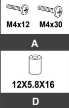
Recessed surface installation: Put 4 spacers between faceplate and monitor. Install 4 screws through faceplate, spacers to monitor via mounting holes.
