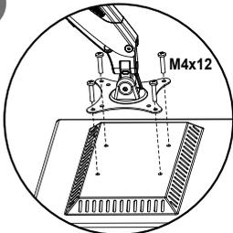
Flush surface installation: Install 4 screws through faceplate to monitor via mounting holes.
