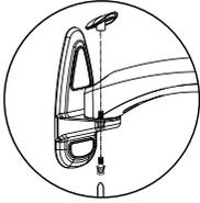
Insert the screw through the hole from the wall plate to the decorative cap.
