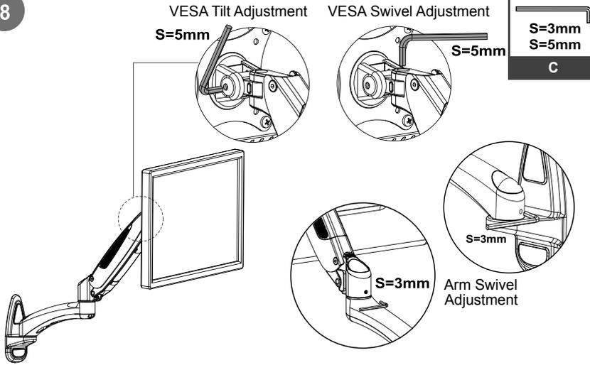
Use a hex wrench to adjust the damp for swiveling. Turn counter-clockwise to reduce damping and clockwise to increase damping.
