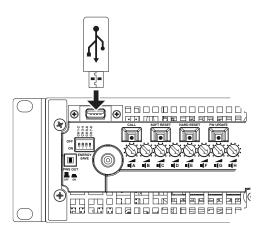
3. Keep pressed the FW UPDATE pushbutton until the front LED bars start blinking.
