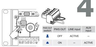
FIG. 3: Manual procedure to switch from LINE to AUX.
