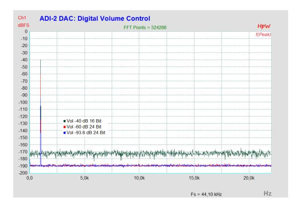
These results clearly show that distortion products of the digital volume control are not drowned by the DAC's noise, but are not generated at all. It works perfectly even with an undithered 16 bit signal, no detectable distortion products are produced.
