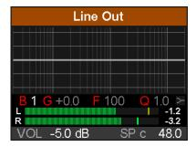
The graph has 5 different colors matching the 5 bands that can be adjusted. If the line is just grey the EQ is disabled (bypass). The EQ can be enabled in the second menu which comes up by pushing the EQ key a second time.
