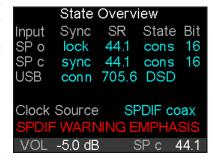
The status bar always shows the current volume setting, the current clock source, and the current sample rate. In case of Sync problems the sample rate will either fluctuate or be shown in red – or both. This information is available in nearly all screens, and helps to get a quick overview of the current state. The State Overview screen now extends this information in great detail.
