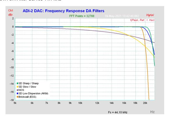
Notes: Sharp/SD Sharp and Slow/SD Slow are congruent. NOS shows a very early drop. SD Low Dispersion only in AKM chip units. Brickwall only in ESS chip units.
