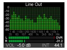
As opposed to most other solutions no FFT (Fast Fourier Transform) is used. RME's Spectral Analyzer performs a true band-pass filter calculation, as in professional hardware devices. The frequency distance between the filters is scaled matching human hearing. The highly optimized code allows to run a 30 band analyzer with 60 dB range, sharp filters and 0.5 dB steps accuracy per band, on the ADI-2 DAC DSP, even at 768 kHz sample rate.
