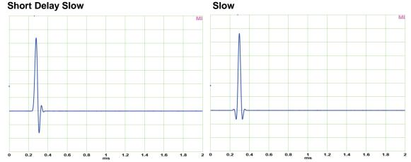
The screenshots above show the analog output signal of the DAC filters, stimulated by a digital single sample impulse at 44.1 kHz sample rate. While Slow has the most perfect response, it looses around 1.2 dB already at 15 kHz, see chapter 31.4. Both Short Delay are IIR filters, the other two are FIR type. FIR is phase linear over the whole frequency range.
