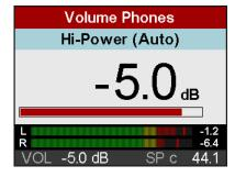
With revised volume settings, where the level meter stays below the red area, the user can now be 100% sure that the ADI-2 DAC operates absolutely free of distortion, even in the most extreme applications.
