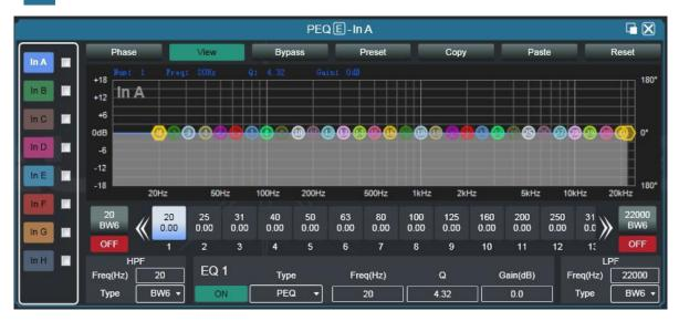
Phase: display the phase curve of the current channel.
