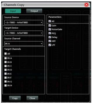
As shown in the figure above, channel copy is to select the channel parameters of one source device and copy them to the target channel of other target devices. Input channels and output channels cannot be copied with each other. The left side is the corresponding channel, and the right side is the copied parameters. The "Input" and "Output" buttons at the top of the interface can switch the channel type of the copy.
