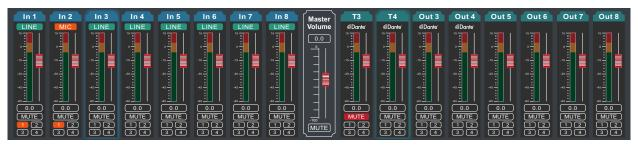
It can display the level, gain, input mode, channel name and other information of each channel, control the main switch of corresponding channel gain and mute, and turn on the group link function of input and output channels, so as to realize more powerful and convenient operation.
