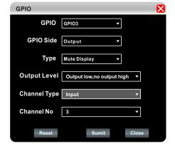
4. For example: when set GPIO side to output, as shown in the right figure, click "Submit" below to make it effective. When the device "system" is set to "mute", GPIO 4 port output low electrical level can be obtained by changing the output electrical level type.
