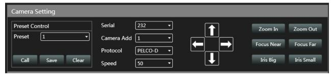
The camera setting is a camera debugging interface. Generally, the camera position is adjusted before the tracking starts, and finally the parameters of this part will remain on the camera.
