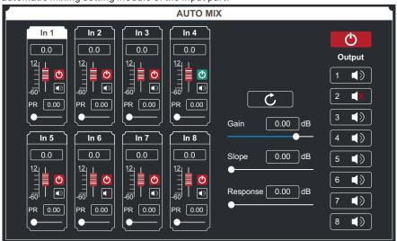
is the input mixing gain of the corresponding channel. Drag the slider or input the corresponding value in the value box at the top; channel input mixing switch and mute switch control whether it is effective (red means off, green means effective); You can adjust the priority of the channel 0-10 to control PR value. The highest priority is level 10.
