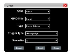
5. For example: when set GPIO side to input, as shown in the left figure, click "Submit" below to make it effective. When the rising edge of GPIO 1 Port is open, call to "archive 1", and the same effect can be obtained by changing the output trigger type.
