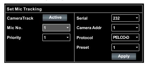
Mic NO. : corresponding to the input channel of the device, that is, the channel number to which the mic is connected. (Parameters need to be set separately for each channel)
