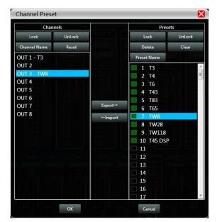
As shown in the picture, there are 8 output channels on the left, you can choose to save the preset for each channel through the "Export" key. You can also load the preset from the right output channel to any other output channel with the "Import" key. Encryption management is available for the presets (only for output EPQ and LIMIT encryption).
