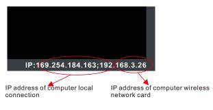
Note: If it is directly connected to the computer through the network cable, please change the IP of the processor to the local IP of the computer and connect it in the same IP segment.
