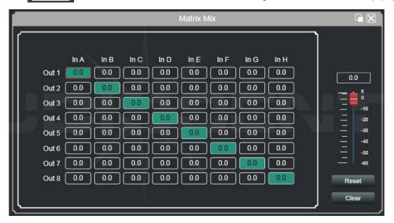
In the figure above, the left is output channel, and the upper is input channel. The value box with the value is the input / output channel mixing key. When the mixing key is green (double-click the value box to switch the state), signals of input and output channel realize the mixing function.
