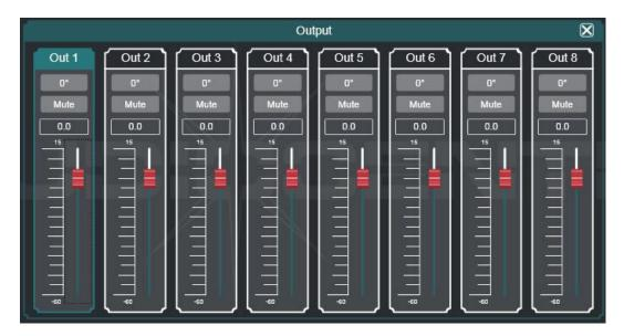
As shown in the figure above, the polarity and mute setting of the corresponding output channel can be controlled.
