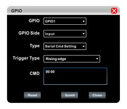
10. For example: when set GPIO side to input, as shown in the left figure, click "Submit" below to make it effective. When the rising edge of GPIO 1 port is opened, the instruction can be sent through 232 port. The same effect can be achieved by changing the content of the instruction.
