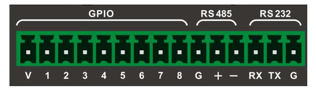
V: means 5V, the internal stabilized voltage output of the device, DC 5V 600mA
