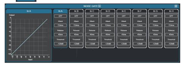
As shown in the figure above, click the noise gate switch to turn on or off the function of the noise gate of the channel. Green means turn on and red means turn off.
