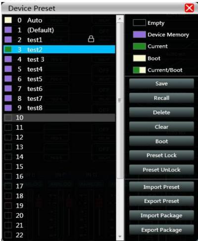
As shown in the figure above, the left side of the archive interface shows gears, where "0 Auto" is the system gear and cannot be used directly; "1 (Default)" is the default gear of the device, which can only be recalled, but cannot be deleted or ovewrritten. After recalling, all the device parameters will be restored to the factory default parameters; other gears can be freely saved, recalled, deleted, etc.
