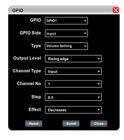
8. For example: when set GPIO side to input, as shown in the left figure, click "Submit" below to make it effective. When the rising edge of GPIO 1 port is opened, the input channel 1 is mute. The same effect can be obtained by changing the trigger type, channel type and channel number.
