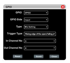
6. For example: when set GPIO side to input, as shown in the left figure, click "Submit" below to make it effective. When the rising edge of GPIO 1 Port is open, the signal of input channel 3 is routed to output channel 4. The same effect can be obtained by changing the output trigger type.
