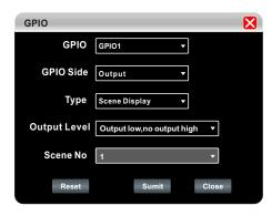
After the device GPIO is connected according to the above method, it needs to be set on the PC as shown on the left. Connect the device in the software, and select Device->GPIO on the menu to start the setting.
