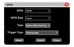
9. For example: when set GPIO side to input, as shown in the left figure, click "Submit" below to make it effective. When the rising edge of GPIO 1 port is opened, the system is mute. The same effect can be obtained by changing the trigger type.
