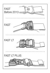
• Check the condition of the DOUBLEBACK adjustment buckles (absence of any deformation, cracks, marks, wear, corrosion).
