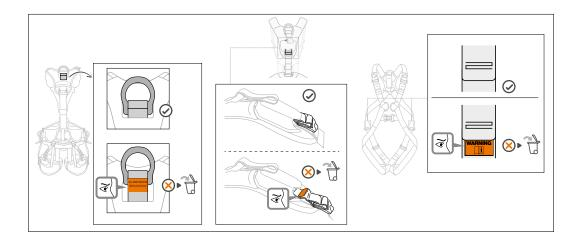
• On the European version of the VOLT harnesses: check the stitching on the LADDER CLIMB attachment-point strap.
