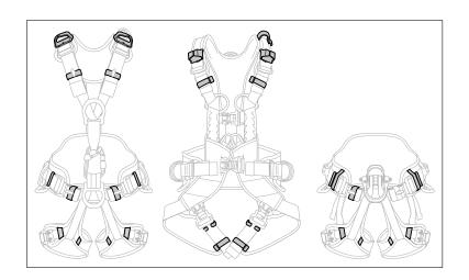
• Check the condition of the equipment loops (e.g. cuts, wear, tears).
