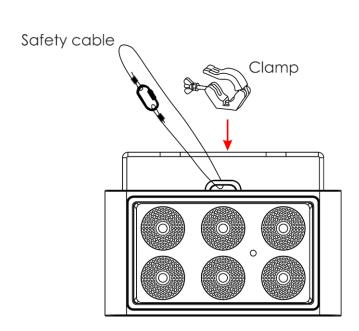
The Cameleon Flood 6WW can be placed on a flat stage floor or mounted to any kind of truss with a clamp.
