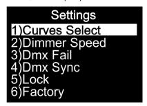
03) Press the **UP/DOWN** buttons to toggle between the following menus: Curves Select, Dimmer Speed, Dmx Fail, Dmx Sync, Lock and Factory.
