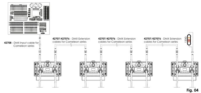
Note: Link all cables before connecting electric power
