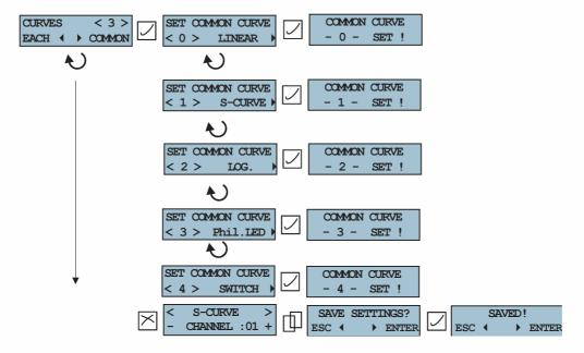
Press the left button to select the curves for each channel individually or the right button to set one common set of curves for all channels.
