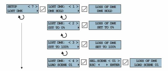
There are four options to set if the DMX signal from DMX port is disconnected:
