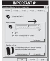
The Windows default output volume setting for USB Audio Devices is 50% of maximum. In many cases this will be too low, inducing noise and hum as excessive gain may need to be applied to deliver the level required. We suggest increasing the output volume setting to 100%.
