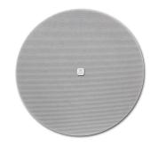
The versatile CMX20DT 8" two-way built-in loudspeaker produces a deep and warm sound ideal for speech and music. When using the loudspeaker at 16 ohms, you can connect up to 4 loudspeakers in parallel on each channel of a standard 4 ohms amplifier.
