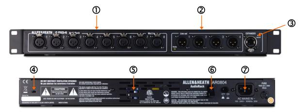
Input sockets 8 balanced XLR inputs for microphone and line level sources. The preamps are built into the AR84 rack and their Gain, Pad and 48V phantom power is remote controlled from the mixer via the digital link. The outputs of the analogue preamps are converted to digital format and transported via a Cat5 cable to be processed and mixed at the mixer.
