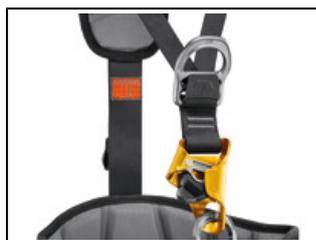
Fall indicator: a red indicator appears on the dorsal attachment point after a fall to signal that the harness should be retired.
