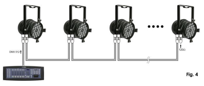
Note : Link all cables before connecting electric power
