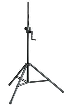
A high quality steel speaker stand with zinc die-cast clamps for professional use. Infinitely variable height adjustment with a hand crank and push button system which prevents an uncontrolled reverse motion. There is an additional locking screw for extra safety. Extension tube diameter 35 mm, suitable for speakers and lighting crossbars with an integrated M10 thread connector.
