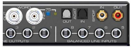
**Word Clock** I/O (BNC): A push switch activates internal termination (75 Ohms). When termination is activated the yellow LED beside the switch lights up.
