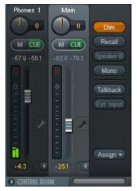
**Speaker B.** Switches playback from Main Out to Main Out B. The faders of the channels Main and Speaker B can be ganged via Link.
