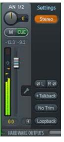
Another difference to the input and playback channels is the **Cue** button instead of Solo. A click on Cue sends the respective Hardware Output's audio to the **Main** Out, or any of the Phones outputs (option *Assign / Cue to* in the Control Room section). With this any hardware output can be controlled and listened to through the monitoring output very conveniently.
