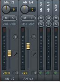
The lowest field shows the current **routing target**. A mouse click opens the routing window to select a routing target. The list shows all activated routings of the current channel by arrows in front of the listed entries, the current one is shown in bold letters.
