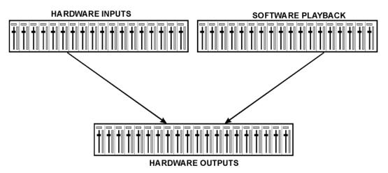
TotalMix can be used in the above view (View Options **2** Row). However, the default is a vertical alignment in three rows as known from an Inline desk, so that the row *Software Playback* equals the *Tape Return* of a real mixing desk:
