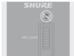
Lower the MIC GAIN if the peak level indicator shows red at any time during a performance.
