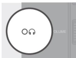
The headphone jack provides direct monitoring of the microphone signal while recording, without any of the delay that occurs if you were to monitor this signal through the computer's headphone output.
