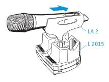
▶ Plug the LA 2 charging adapter with the inserted radio microphone into the L 2015 charger (see "Accessories and spare parts" on page 31).
