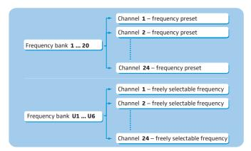
Each of the channels in the frequency banks "1" to "20" has been factory-preset to a fixed frequency (frequency preset).
