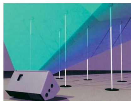
Figure #2: (Above) With horn rotated 180° from Figure #1, this monitor application provides a wide (100°) sweet spot for the performer's listening zones, and restricts unwanted below-the-belt coverage.
