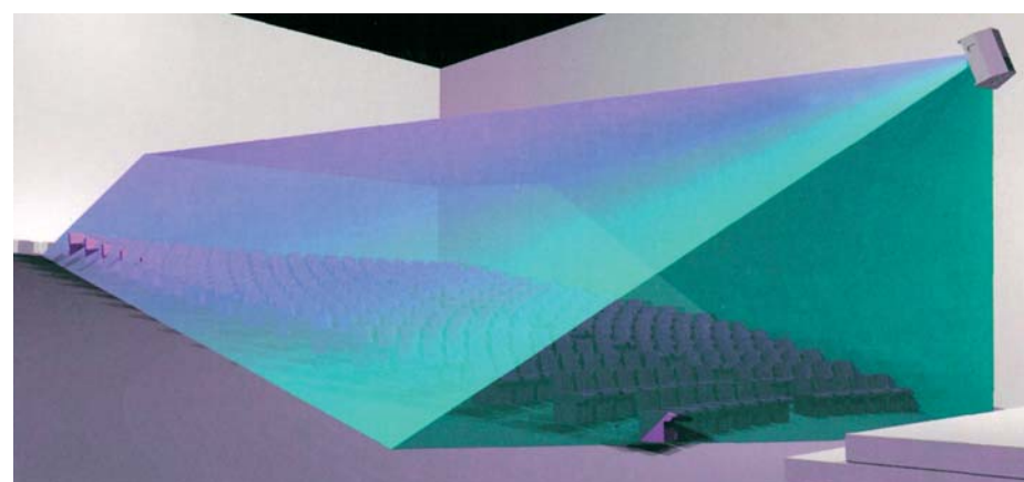
Figure #1: (Above) Computer representation of how the PS Series' asymmetrical horns match pattern control to the seating area of a typical rectangular venue.
