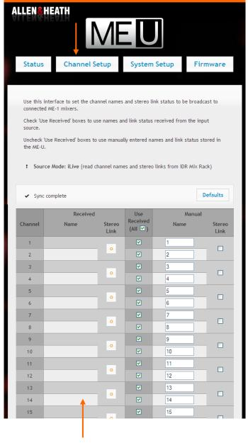
This example shows no name and stereo link data received. This is the default on power up when no input is connected, or when you are working with a source that does not broadcast the channel data.
