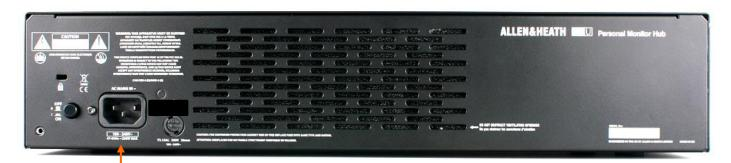
Main Input - IEC connector, fuse and ON/OFF push switch for the built-in universal voltage power supply unit. This accepts worldwide voltages from 100 to 240V AC 50/60Hz. Check that you have received the correct mains lead for your territory.
