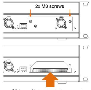
Slide card in to plug into connector
