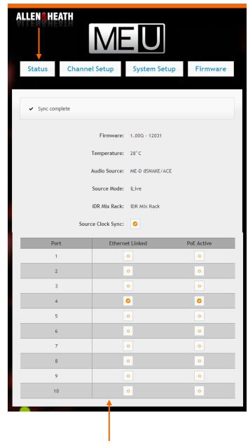
Port Status - Displays the current connection status of each of the 10 output ports:
