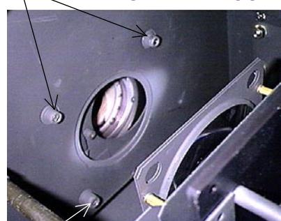
*Adjusting stopper for positioning.*
