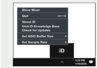
Once installed, the iD mixer can be opened by going to the system tray and right clicking the iD icon
