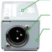
**GROUND LIFT** - Disconnects PIN-1 on the XLR output to eliminate hum and buzz created by ground loops.
