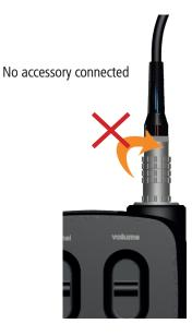
Use the "Mic" icon on the terminal screen to make sure that the headset is properly connected. After disconnection of a headset, it is necessary to wait a few moments for the mic icon to be crossed out before reconnecting a headset.
