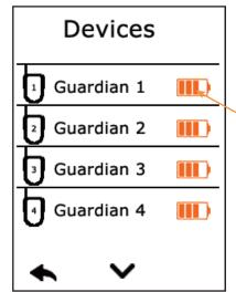
This screen indicates the terminals present on the configurator. The charge status as well as the name of each terminal displays. The terminals display in their order of presence on the configurator, going from the closest (position 1) to the furthest away.
