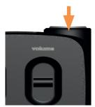
Plug the headset into the LEMO connector at the top end of the product, beside the LCD.
