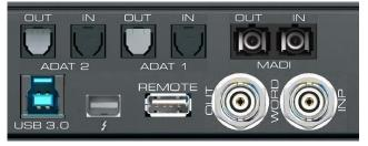
**Word Clock I/O.** BNC. In the Settings dialog, Input Options, this input can be set to be terminated with 75 Ohms internally.
