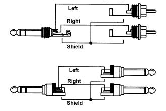
The pin assignment follows international standards. The left channel is connected to the tip, the right channel to the ring of the TRS jack/plug.
