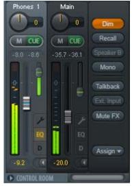
Mono. Mixes left and right channel. Useful to check for mono compatibility and phase problems.
