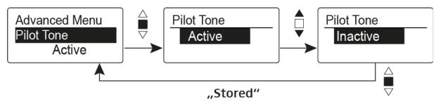
The pilot tone has an inaudible frequency that is sent from the transmitter and evaluated by the receiver. It supports the receiver's squelch function.
