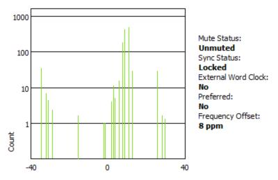
A histogram that shows measurements in amber and/or red indicates a clock that might be *currently* stable, but has little room for manoeuvre; its offset could easily move outside its pull range, at which point it will lose sync completely. This can result when the master clock is derived from an inaccurate external word clock.
