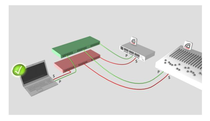
**Note:** You must be connected to a standard wired Ethernet network in order to use Dante Controller. Wireless and other non-standard wired Ethernet interfaces will not appear in the Configure Dante Interfaces dialog.
