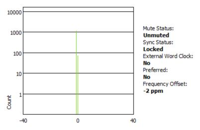
A histogram that shows a distributed range of offsets indicates an unstable clock - it is having to change its offset significantly, and often, to stay in sync with the master clock. This can be due to overloaded network links, or poorly-implemented EEE. A device in this state is highly likely to lose sync with the master clock.
