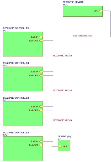
During operation, the NC4MXX plug must be connected to the last controller in chain
