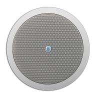
The Apart CM6T is a 2-way 100V/70V/16 ohm built-in ceiling loudspeaker. The loudspeaker has a 6½" woofer, a 1" coaxial tweeter and a high quality 100/70 volt speaker line transformer with multiple power taps. It's the perfect choice for the distribution of microphone calls and background music. The mounting frame is made of high quality ABS. The grille is made of aluminium.
