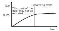
Also remember that when recording from an analog source, the threshold should be set so that it is higher than the "noise floor". If the "noise floor" is higher than the threshold, a false start will occur:
