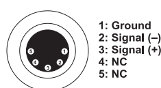
DMX-output XLR mounting-socket:
