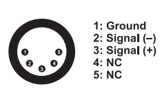
DMX-input XLR mounting-plug:
