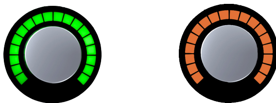
Arrow's top panel preamp knob during normal operation (left) and when a Unison plug-in is in the Unison insert of Arrow's selected channel (right)
